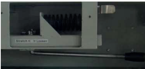
Hefboom om de band te spannen of losmaken
