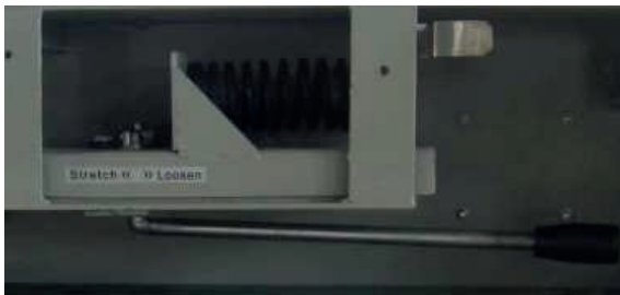
Belt tension release lever
