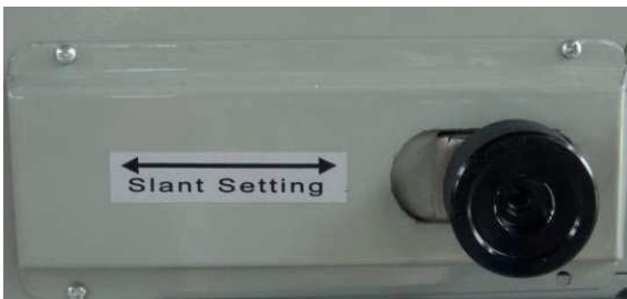
Belt deviation adjustment handle
